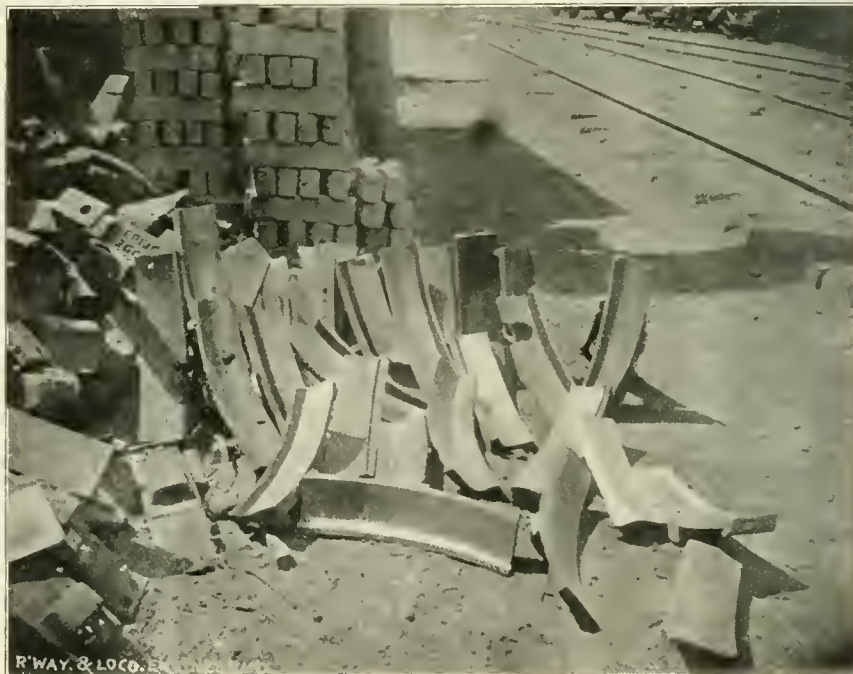
SCRAP HEAP SHOES, SHOWING UNEVEN WEAR, DUE TO TOO GREAT DISTANCE BETWEEN BRAKE SHOE HEADS.
